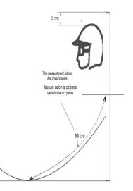
The structure in all open cars must be a minimum of 5 cm above the top of the driver's and co-drivers helmets at all times.
